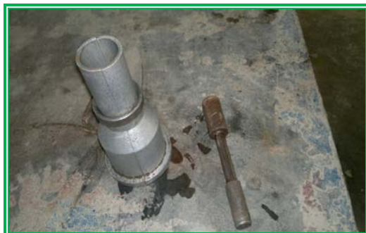
Plate (1) Mold & manual hammer used in UCS
