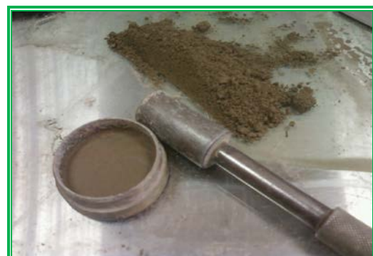
Plate (3) Sample preparation for swelling and consolidation tests
